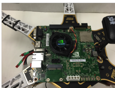
Figure 6: Original Hexacopter with NVIDIA GPU-enabled Design
