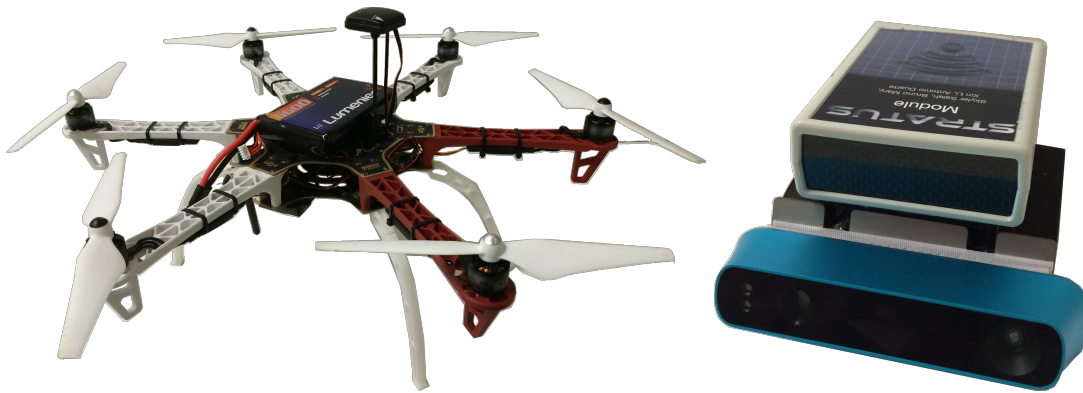
Figure 5: Stratus Module Deployment in Hexacopter and Mini-Rover Platforms
