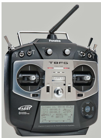
Figure 17: Radio Transmission Controller
